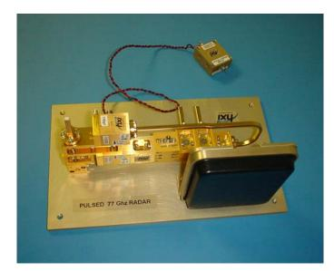
77 GHz Pulsed Radar Prototype for Intelligent Cruise Control Applications
